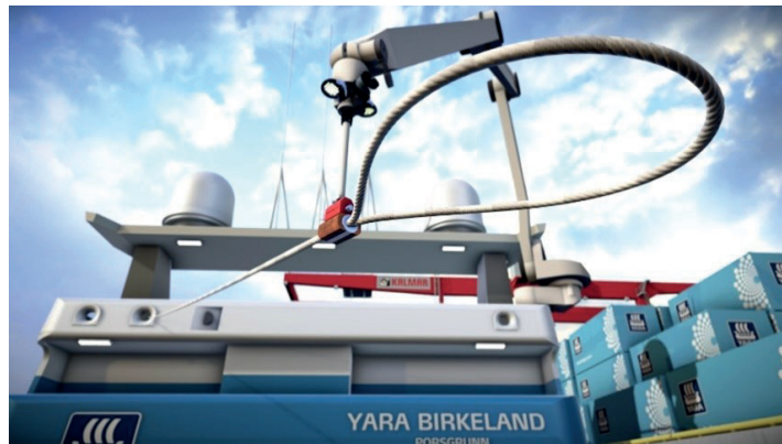
Figure 1: Illustration of the autonomous mooring system
